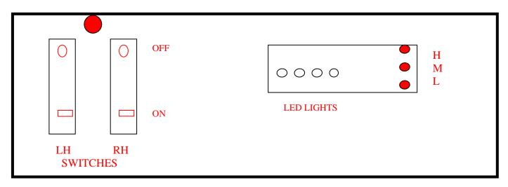
To operate on HIGH – switch BOTH switches on (down) – heater will start up in a few minutes.
